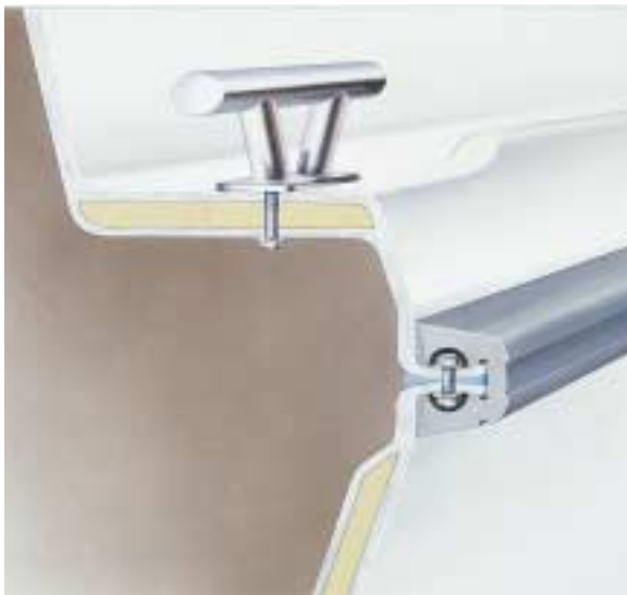
Robust rubbing strake in PVC and sandwich hull.
