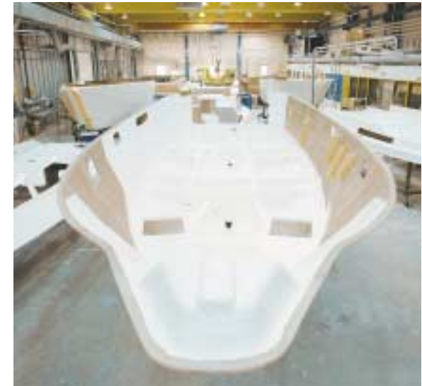
Innerliner in fibreglass means superior rigidity with a high degree of maintenance-free finish.
