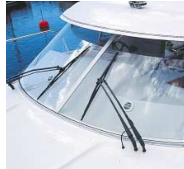
Curved windscreens in tempered glass with powerful windshield wipers.
